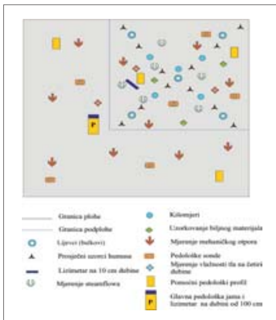
Slika 4. plohe s mjestima uzorkovanja i instrumentima za praćenje Figure 4 Rough draft of the plot with sites of sampling and instruments for monitoring
